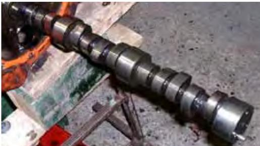
V-8 engines with flat tappets are particularly susceptible to failure, or maybe it just appears that way because there are more of them, but a lot of failures have been reported.<sup>5,6,7</sup> These engines provided long service life with the old oil formulations they were designed for, but failure rates have increased with today's low-phosphorus passenger car motor oils.
