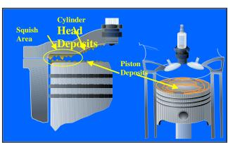
Cen-Pe-Co Gas-O-Klenz removes combustion chamber deposits, allowing the engine to operate more efficiently and on lower octane gasoline.
