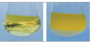
Phase Separation happens when ethanol blended fuels pick-up more water than the ethanol can absorb, reaching its saturation point. At this time (as shown on the right) the ethanol and water will separate, actually coming out of solution and forming two distinct layers in the tank.
